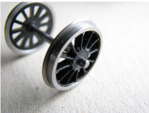
Gibson wheels mounted onto new 2mm axles.
