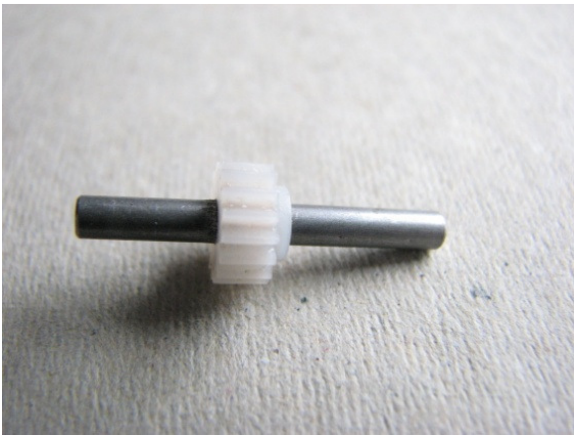
Gear on new axle – note boss faces chassis centre.
