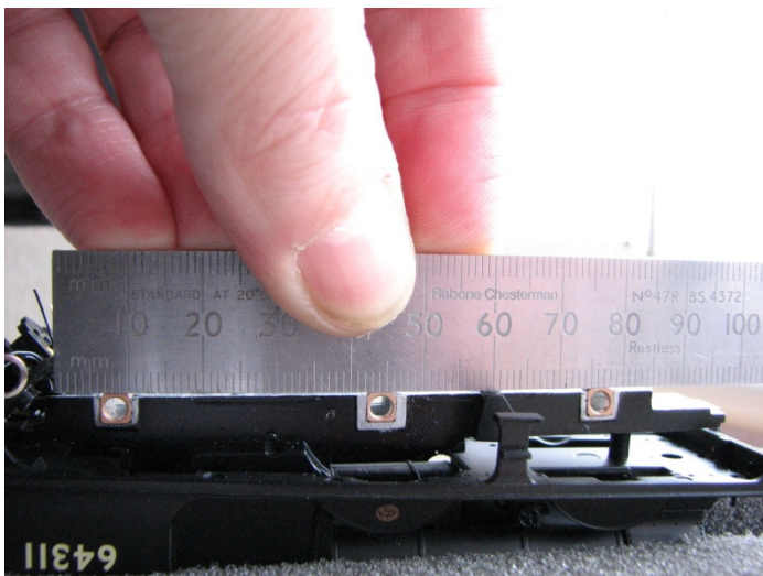
Checking axle heights.
